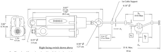
$F_T$ = The value of force, along the cable, which trips the switch.
